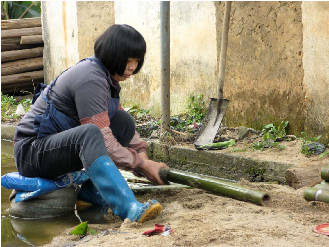
Fig. 10 Removal of the natural wax layer with sand and water.
