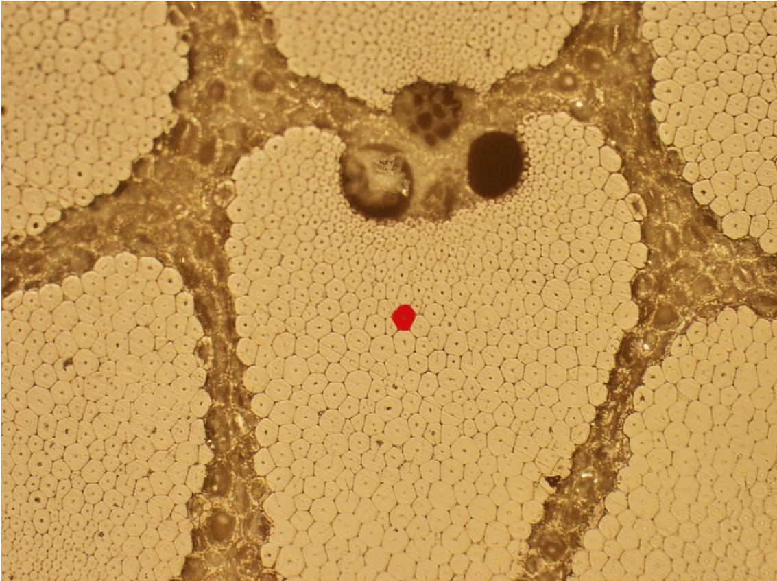
Fig. 2 Cross-section of a fibre bundle of Chinese Tonkin. Single fibre marked in red is 0.03 mm across.
